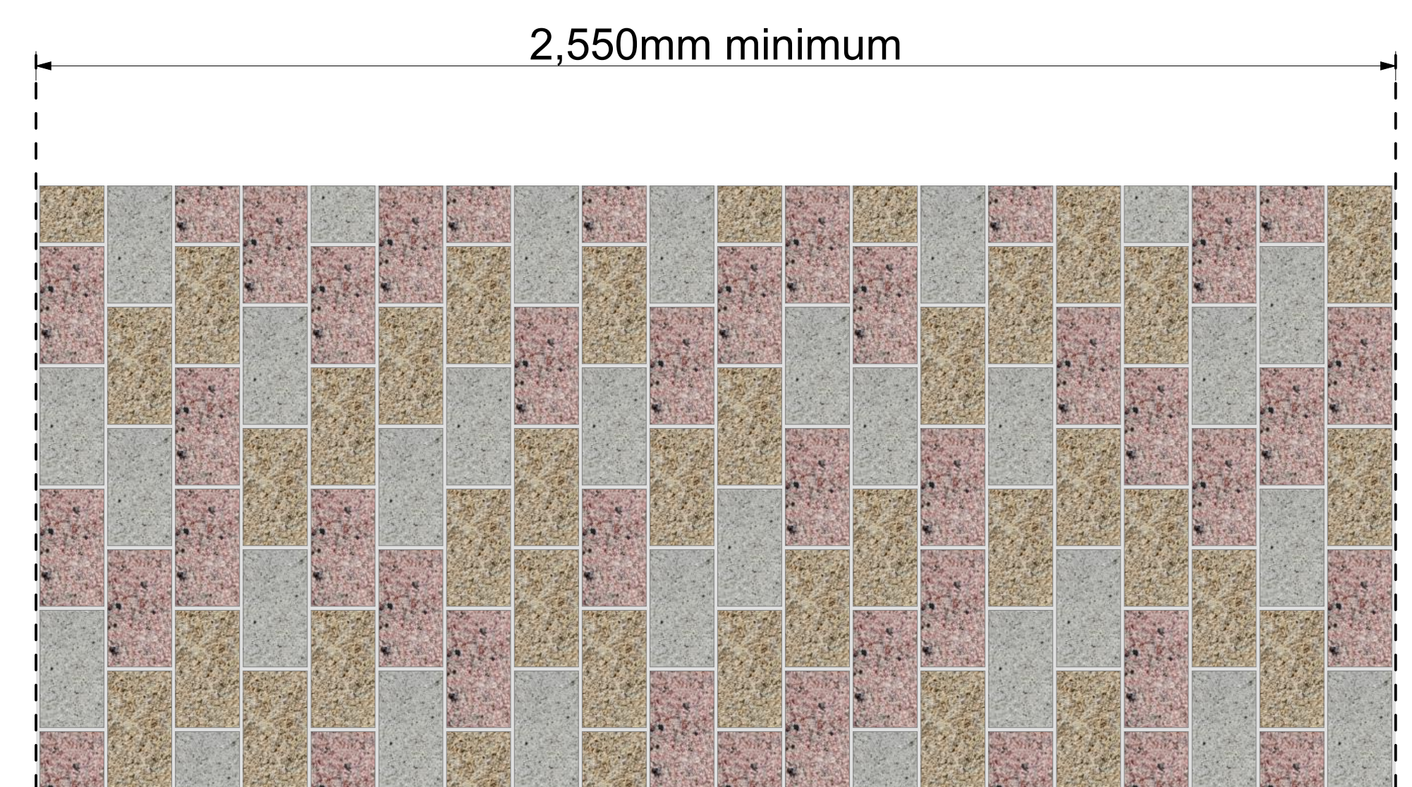
Randomised grey, pink and buff 120mm x 220mm granite sett paving to identify and give warning of pedestrian intersections
